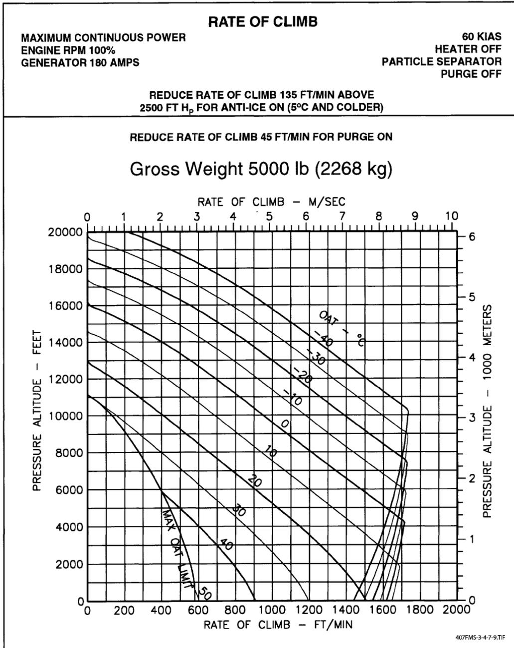
Figure 4-11. Rate of Climb — Maximum Continuous Power (Sheet 9 of 10)
