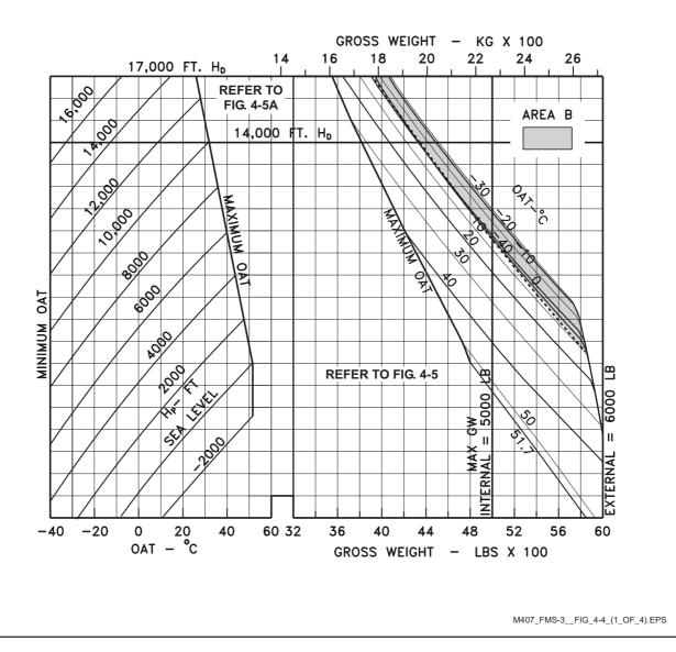
Figure 4-4. Hover ceiling OGE – takeoff power (sheet 1 of 4)
